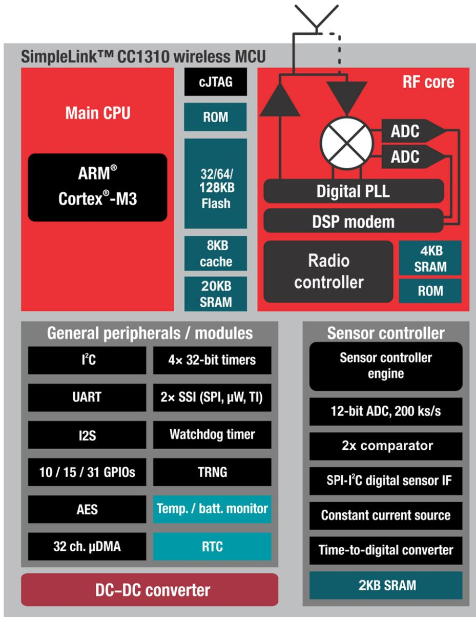
Figure 1-1. CC1310 Block Diagram
